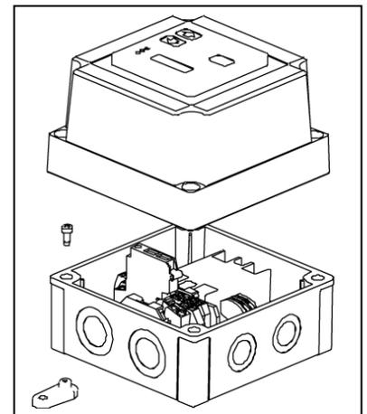
5. Thread the (3) wires and the thermocouple through the drilled hole. The foam sealing washer should be placed on the outside of your electrical enclosure between the liquid tight conduit connector and the metal enclosure. Tighten the retaining nut from the inside of the enclosure to ensure a tight seal at the foam washer.
