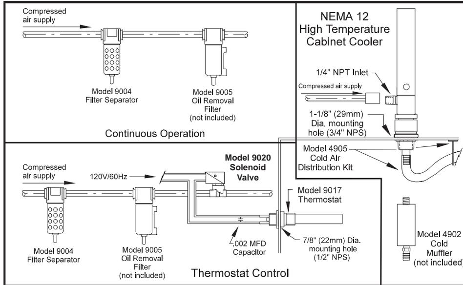
**High Temperature Cabinet Coolers are rated for a maximum temperature of 200°F (93°C)**
