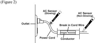
As you move the plastic probe tip away from the electrical source (in this case the wall receptacle), the probe tip will stop glowing at the exact break point in the wire. (Figure 2)
