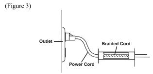
Round electrical cords that contain a twisted conductor internally will cause the AC Sensor to glow, stop glowing, then glow again as the probe tip is moved along the length of the cord. This is due to the spiral of the conductor wire that produces voltage. (Figure 3)
