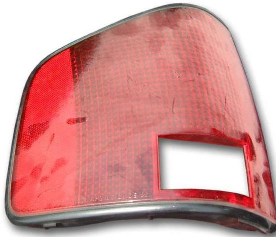
Normally three major parts make up any lighting unit; the reflector lens which is also the rear housing, the lens cover (shown above) and the electrical components. There are at least three potential applications common to lighting manufacturers depending on the “local styles” and manufacturing process, but there can be more.
