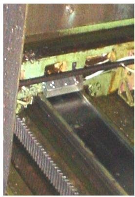
Six EXAIR Super Air Knives Model BP110006 were mounted on the carriage (three each side) above the slide and guide ways. The Super Air Knives completely covered the six individual slide ways with a uniform sheet of high velocity air so the chips would be blown off as the carriage of the machine was moved.
