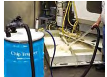
The Chip Trapper pumps the coolant back into the sump – free of chips and debris.
