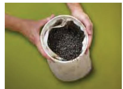
The 5 micron filter bag traps all the chips so no solids get pumped back out of the drum.
